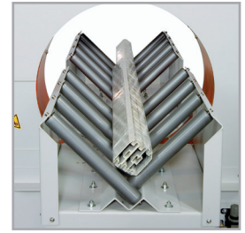
VERTICAL PRESSURE WITH FREE ROLLER FOR A MANUAL ADJUSTMENT
